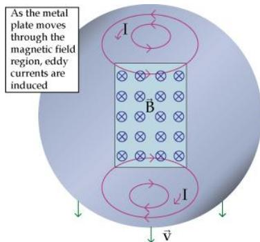
**Figure 3. Eddy current formation (Courtesy of Das)**
