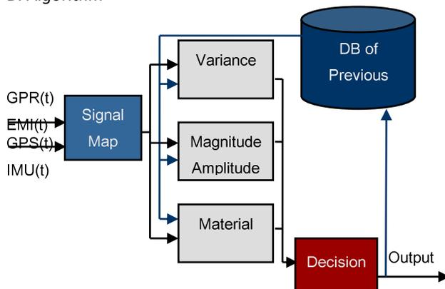
**Figure 4. Block diagram of algorithm**
